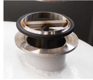
Step c : centering ring removal
