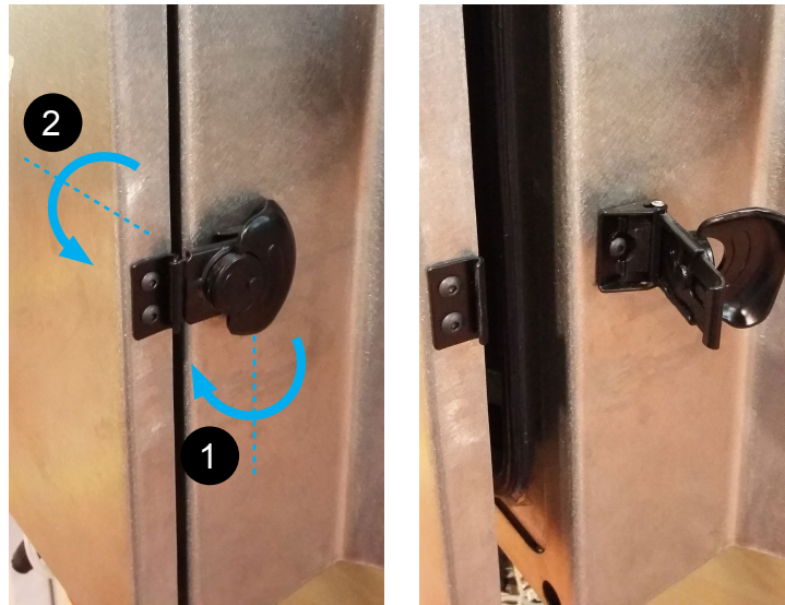
Airlock door closed and locked.
