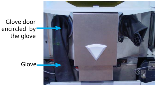
Good gloves position before front doors closure.
