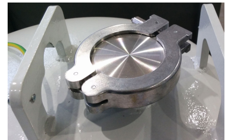
Step c : clamp tightening
